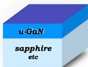
Typical Epi Structure
